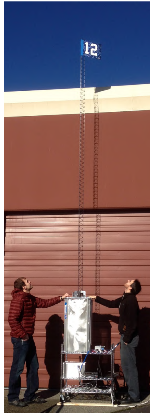
Caption: TUI’s “Trusselator” technology enables on-orbit additive construction of high-performance composite truss structures to support solar arrays, antennas, and other space system components.
