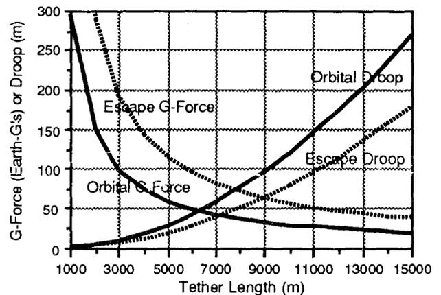
Figure 3 Tether Droop and Payload G-force vs Tether Length
