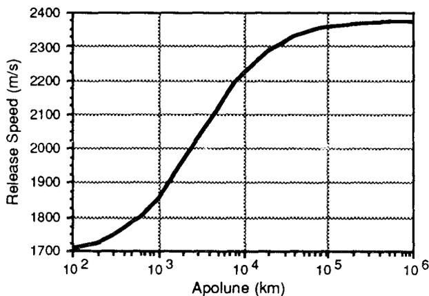
Figure 2 Apolune Altitude vs Release Speed for Captured Lunar Orbits
