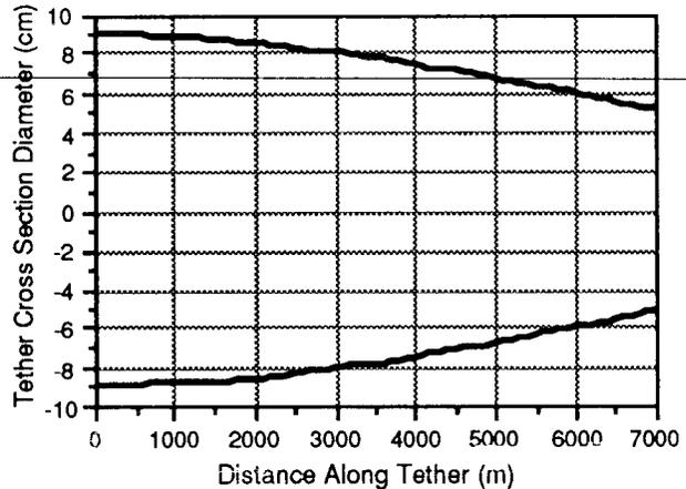
Figure 5 Tether Diameter vs Length
