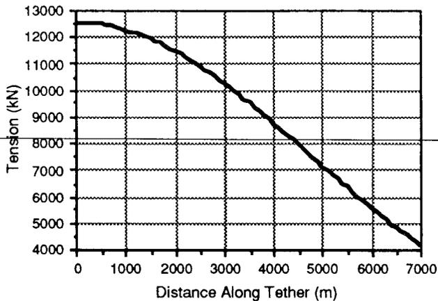
Figure 4 Tether Tension vs Length
