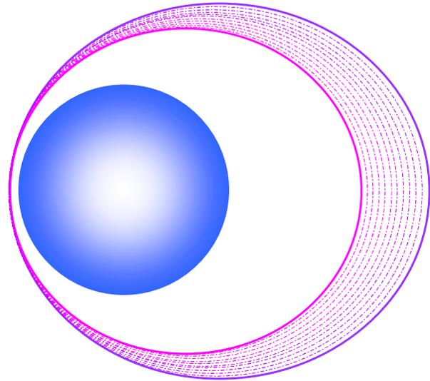
**Figure 2: Electrodynamic reboost centered on an arc about perigee can be used to boost apogee and restore orbital energy.**
