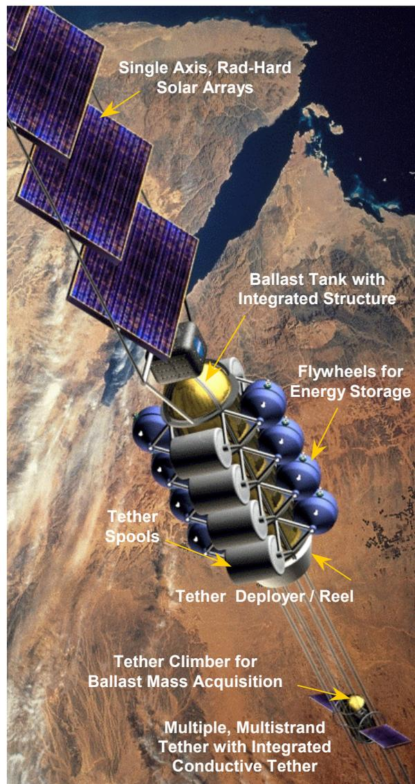
**Figure 4: Conceptual configuration of a modular tether station demonstrating power collection, energy storage, staged tether deployment, and allocation for ballast mass collection.**
