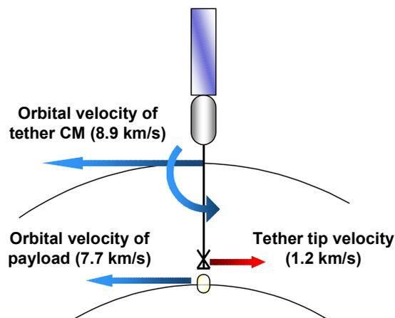
**Figure 3: The tip velocity of the tether is configured to be equal to the difference in orbital velocity between the tether and payload, enabling them to match position and velocity instantaneously.**
