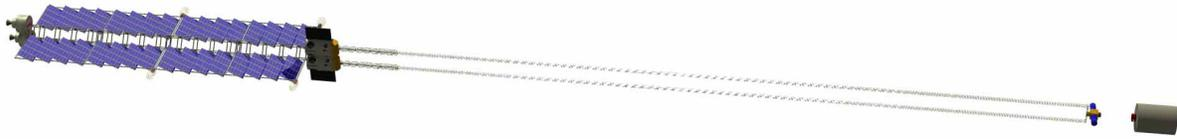
**Figure 5.** Tether Boost Facility with two modules, capable of tossing 5000 kg to GTO and 2000 kg to LTO. (Tether length not to scale)
