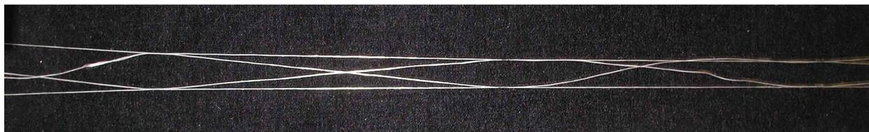
**Figure 2.** A section of conducting Hoytether™ constructed of metalized Kevlar.®
