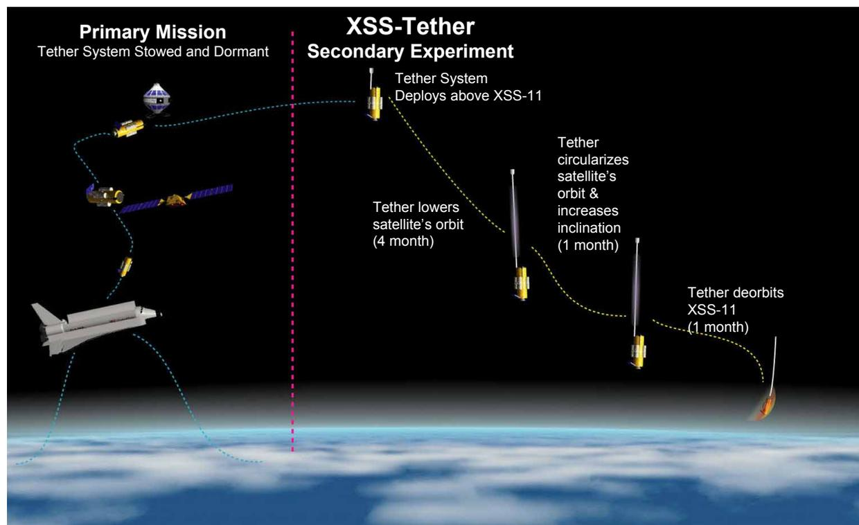
FIGURE 1. The proposed Microsatellite Tether Deorbit Experiment concept.
