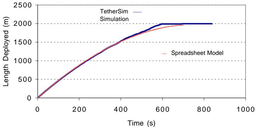
**Figure 6.** Results of a deployment simulated using TetherSim and the drag vs speed characteristics given in Figure 5 with an endmass ejection velocity of 5 m/s.
