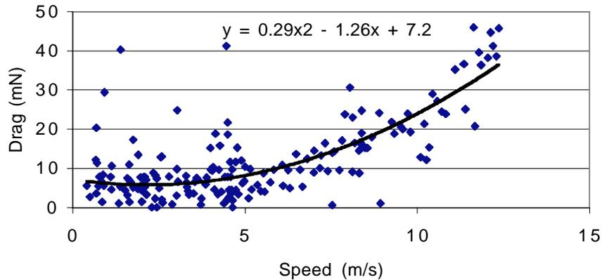
**Figure 5.** Deployment Drag vs. Deployment Speed for a tether constructed of metalized Kevlar®, deployed from a 1” diameter spool, 3” winding OD, with a smooth 3.5” ID shroud.
