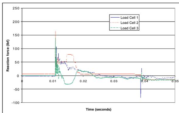
**Figure 7.** Reaction force data measured by the three load cells
