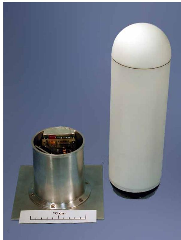
**Figure 4.** The prototype RETRIEVE avionics and deployer.
