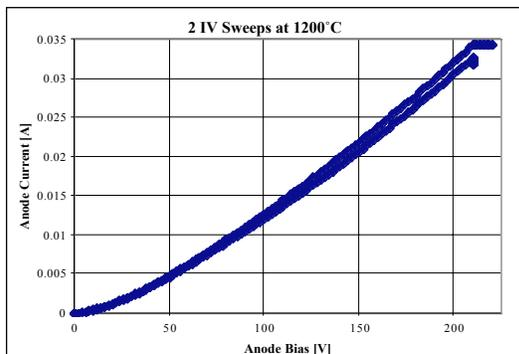
**Figure 10.** Current-Voltage characteristics of the thermionic emitter, without accelerating structures.
