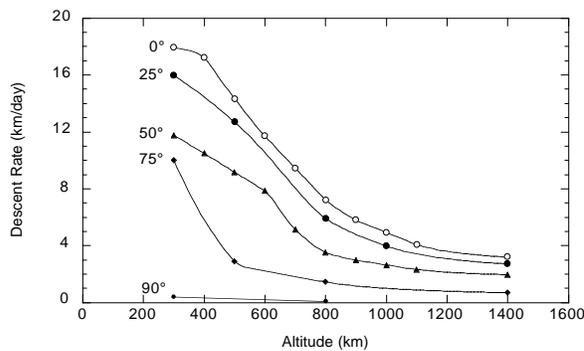
**Figure 18.** Rate of descent for a 7.5 km, 15 kg aluminum tether with a 15 kg endmass, deorbiting a 1500 kg spacecraft at various inclinations and altitudes.
