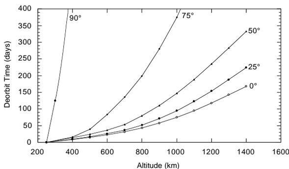
**Figure 19.** Time for a Terminator Tether™ with a 7.5 km, 15 kg aluminum tether and 15 kg endmass to decrease the perigee altitude of a 1500 kg spacecraft to 250 km. Note that deorbit time can be decreased by using longer or more massive tethers.
