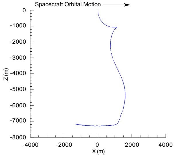
Figure 11. Deployment of the tether from the Terminator Tether™, with segmented tether model.
