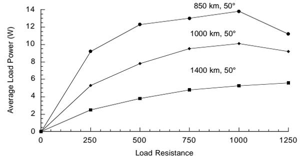
**Figure 9.** Average load power over one orbit as a function of series load resistance for the 5 km tether.
