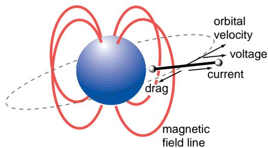
Figure 2. Electrodynamic tether drag.
