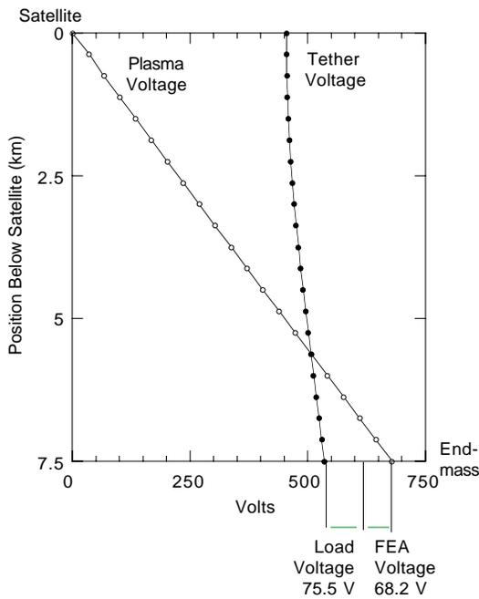
**Figure 6.** Tether and plasma voltage for a 7.5 km, 15 kg Terminator Tether hanging below a satellite in a 850 km, 50° inclination orbit, with a 250 ohm load resistance.
