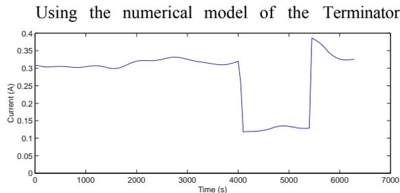
**Figure 8.** Tether current over one orbit for a 10 km, 15 kg tether deployed from a spacecraft in a 1000 km, 50° orbit with a load resistance of 250 Ω.
