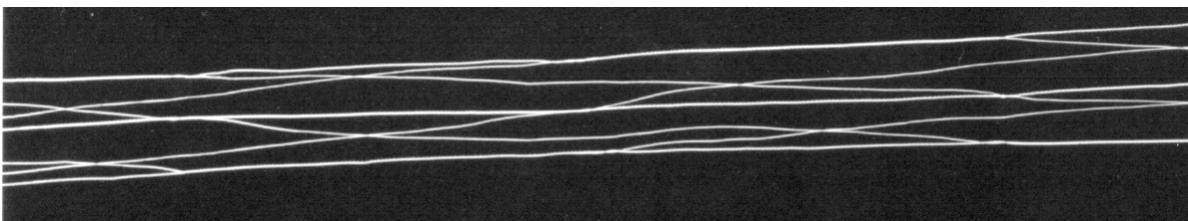
Figure 3. Photo of a 20-cm length of the conducting Tri-Line Hoytaper made of 30 gauge aluminum wires knitted together with 22-Tex P.T.F.E. thread.
