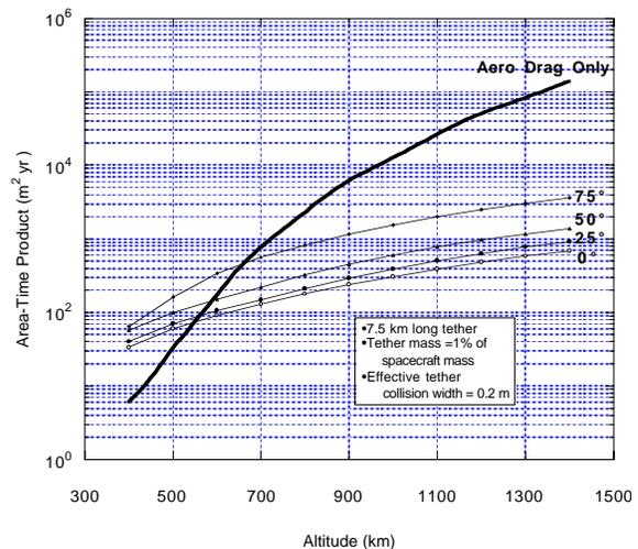
**Figure 20.** Area-Time-Product for Terminator Tether™ systems with tethers massing 1% of the host spacecraft mass, compared to the ATP for deorbit of the host spacecraft due to aerodynamic drag alone.
