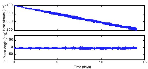
**Figure 17.** Host spacecraft altitude and tether in-plane libration angle with feedback control on the in-plane libration. The feedback succeeds in keeping the tether dynamics under control.
