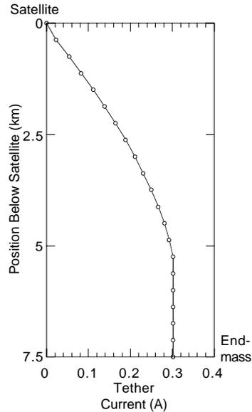
**Figure 7.** Tether current as a function of distance below the host satellite.
