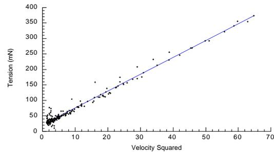
Figure 13. Plot of deployment tension versus the square of the deployment speed for the Spectra Hoytether paying out from the SEDS deployer with no braking applied.
