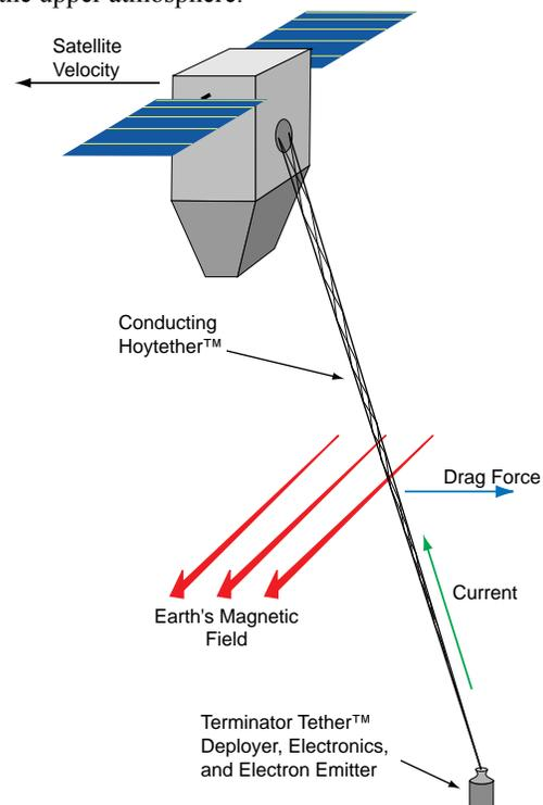
Figure 1. The Terminator Tether™.
