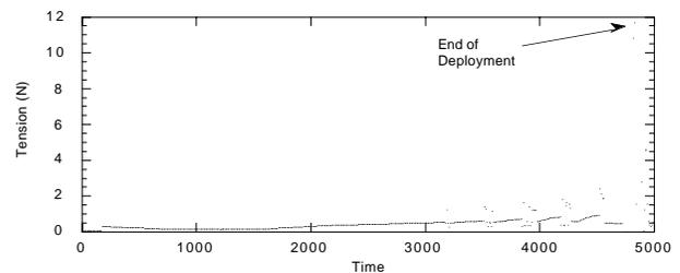
Figure 14. Tension experienced at the endmass, with segmented tether model.
