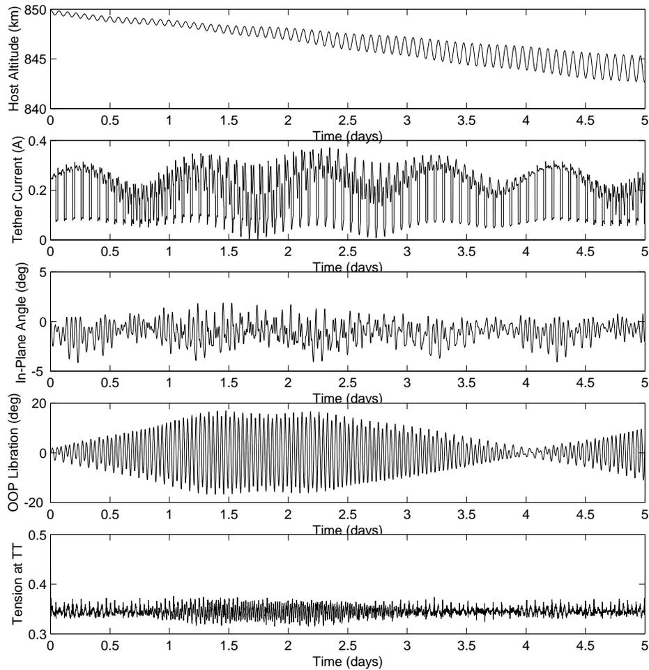
**Figure 15.** Data for a 5-day simulation of a Terminator Tether starting in a 850 km, 50° initial orbit.
