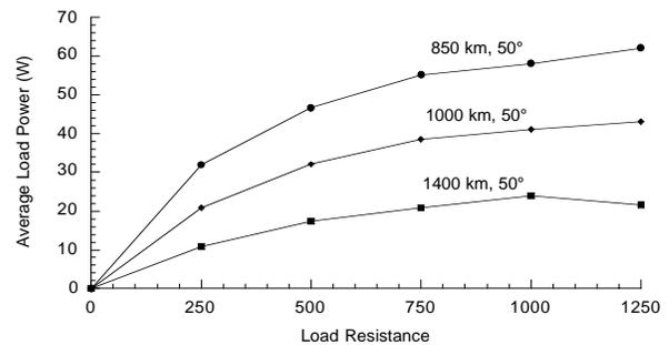
**Figure 10** Average load power as a function of series load resistance for a 15 kg, 10 km aluminum tether.
