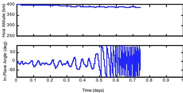
**Figure 16** Host spacecraft altitude and the in-plane libration angle of the tether endmass for a 15 kg, 7.5 km long tether deorbiting a satellite from a 400 km, 50° inclination orbit with no feedback control.
