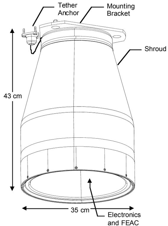
Figure 4. Schematic of the Terminator Tether™ Assembly.
