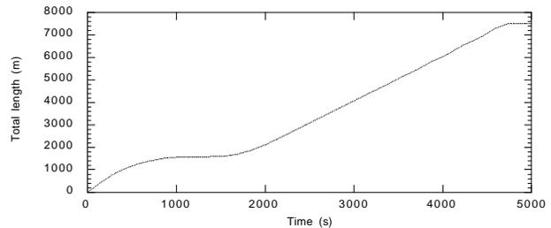
Figure 12. Deployed length as a function of time with segmented tether model.
