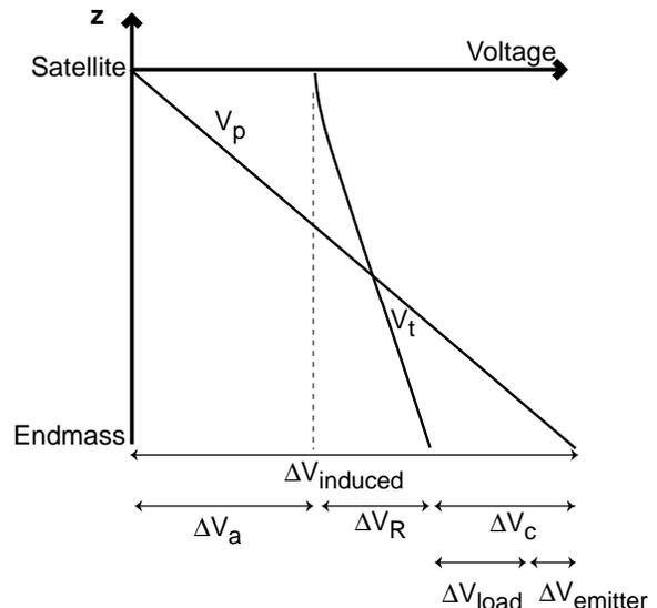
**Figure 5.** Tether voltage and plasma voltage along the tether length.
